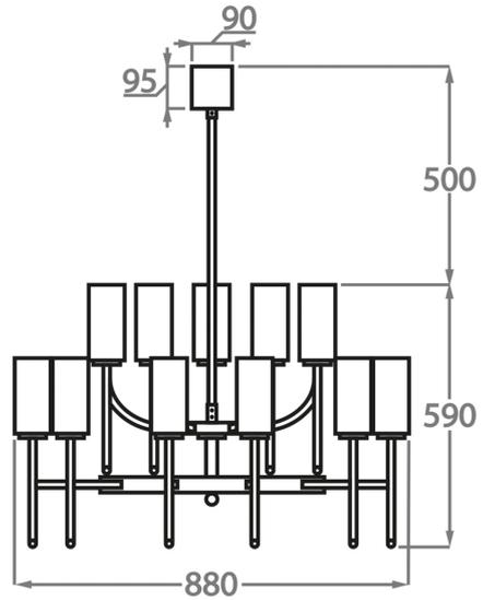
The dimensions of the central rod/chain and ceiling rose are not included in the height measurements.
