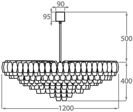
The dimensions of the central rod/chain and ceiling rose are not included in the height measurements
