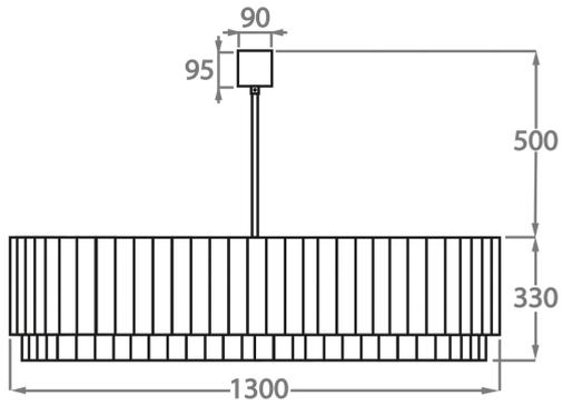
The dimensions of the central rod/chain and ceiling rose are not included in the height measurements.
