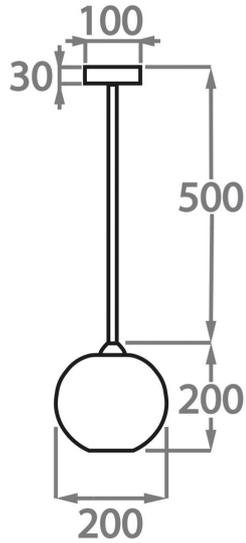
The dimensions of the central supporting rod and ceiling rose are not included in the height measurements
