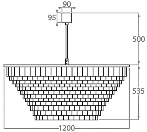
The dimensions of the central supporting rod and ceiling rose are not included in the height measurements.
