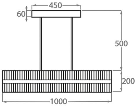
The dimensions of the supporting rods and ceiling rose are not included in the height measurements.
