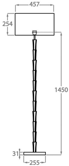
Dimensions are measured from the base of the lamp to the middle of the bulb holder and are excluding shade
